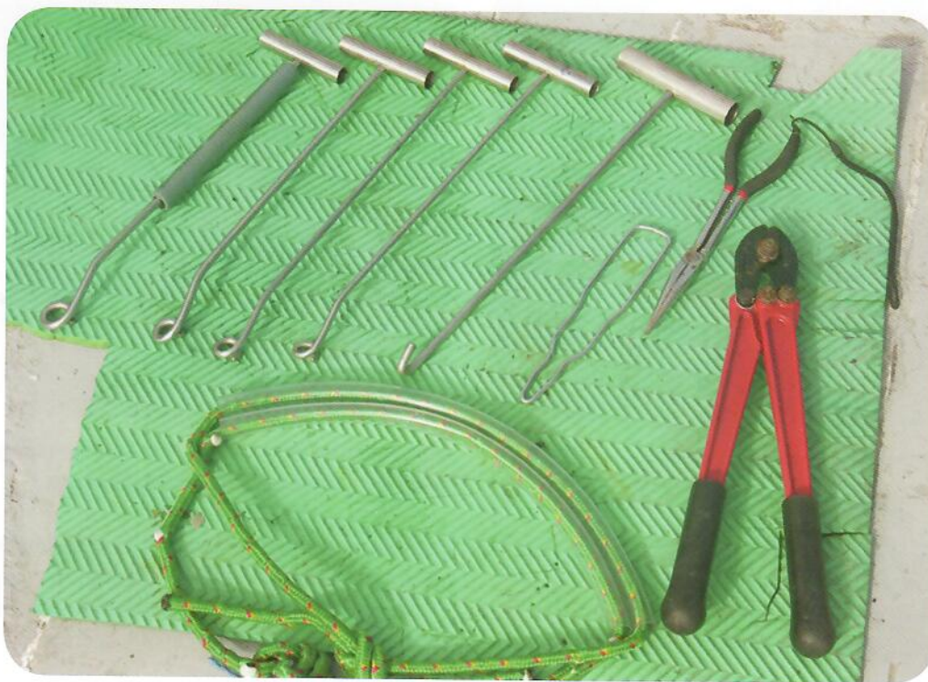
De-hooking and line cutting equipment that can be used to safely release a sea turtle that is accidentally captured during longline fishing operations.
