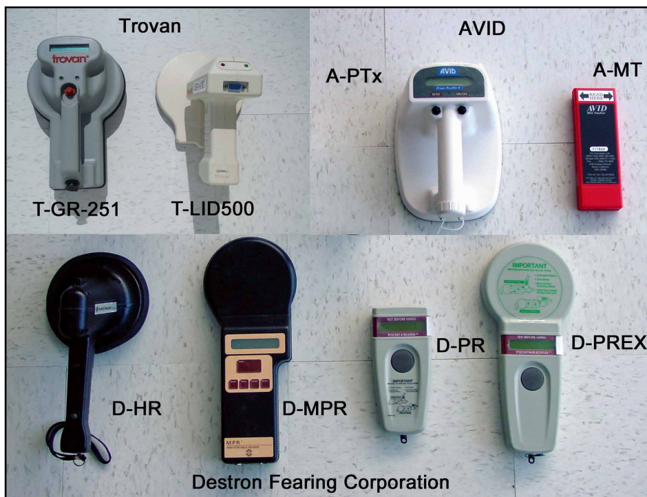
Figure 2. Portable RFID readers tested: Trovan GR-251 and LID-500, AVID Power Trackers and MiniTracker, and Destron Fearing Handi Reader, Mini Portable Reader, Pocket Reader, and Pocket Reader EX.
