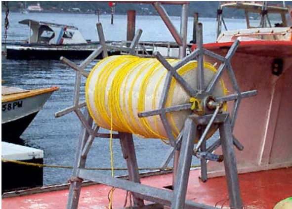
Figure 27.—Hand cranked mainline reel on an alia .
