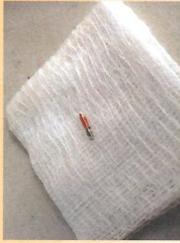
PIT tags are small microchips about the size of a grain of rice.
