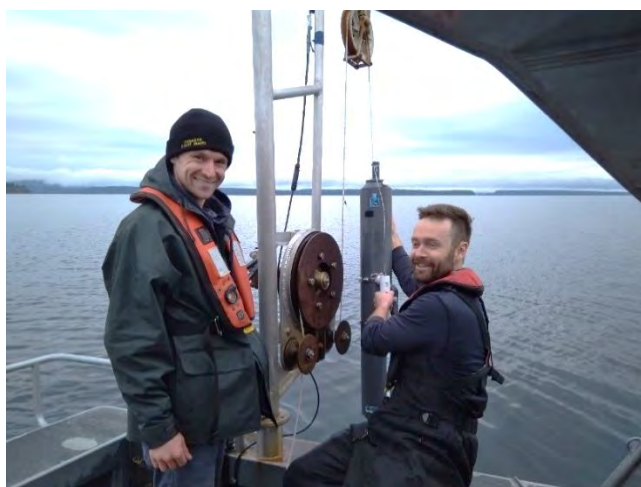
Chris Mackenzie and Brett Johnson (Hakai Institute) showing participants how to deploy Niskin bottles for water sampling.
