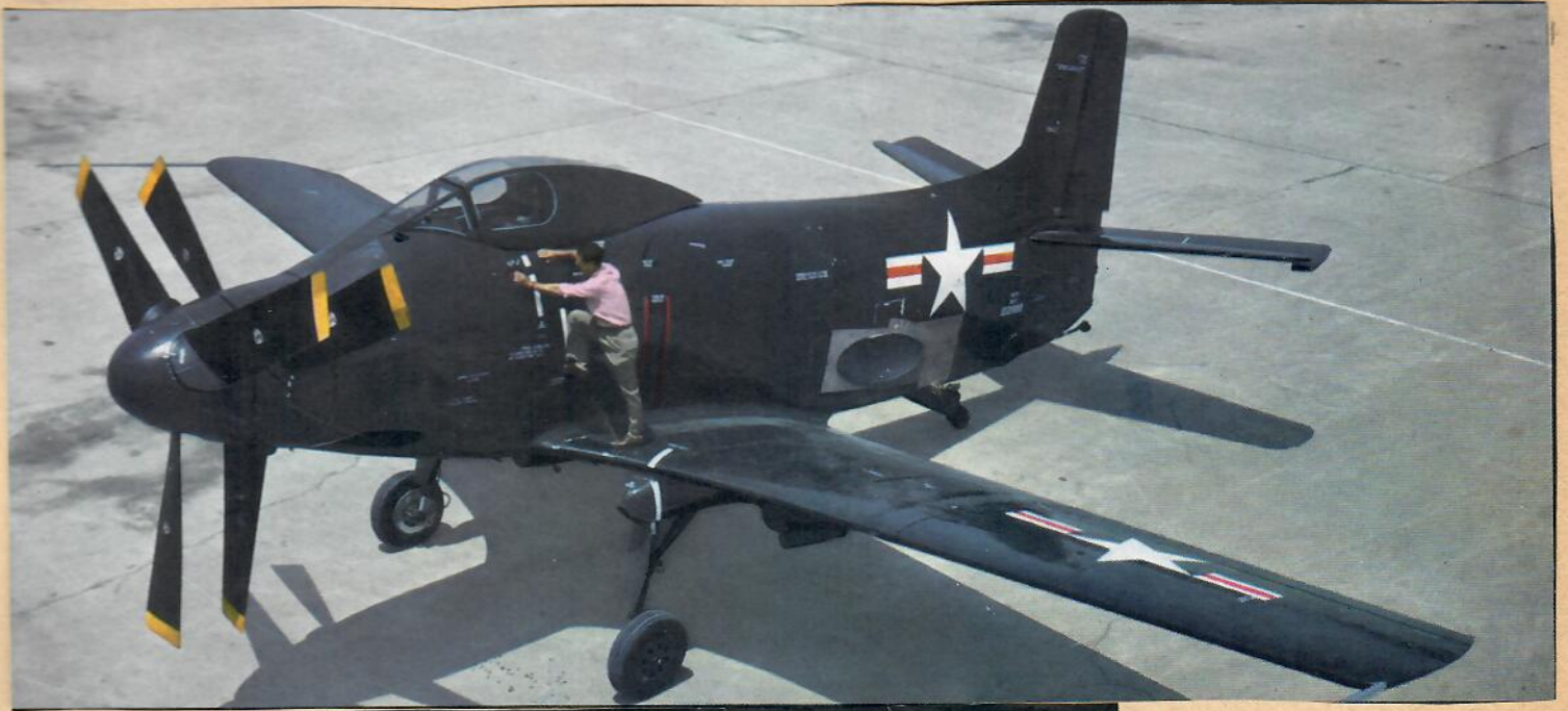
▲ A2D Skyshark has propellers driven by two jet turbines.
