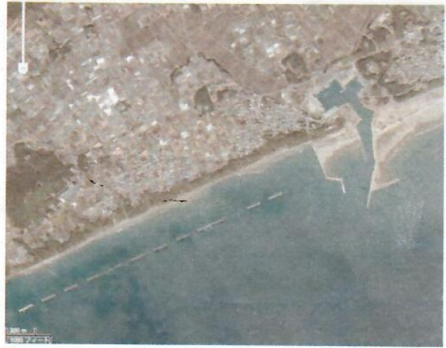
Figure 2. Aerial view of northeastern Omoteshama showing nearshore armoring structures. All photos courtesy of Y. Tanaka, Omoteshama Network
