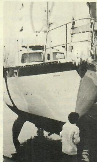
TWA pilot John Traylor of Los Angeles USA designed and built the 13 m foam-core twin-keel sloop Beyond seen here being lifted from the water. One of the twin keels is shown clear of the water. — John Traylor picture.
