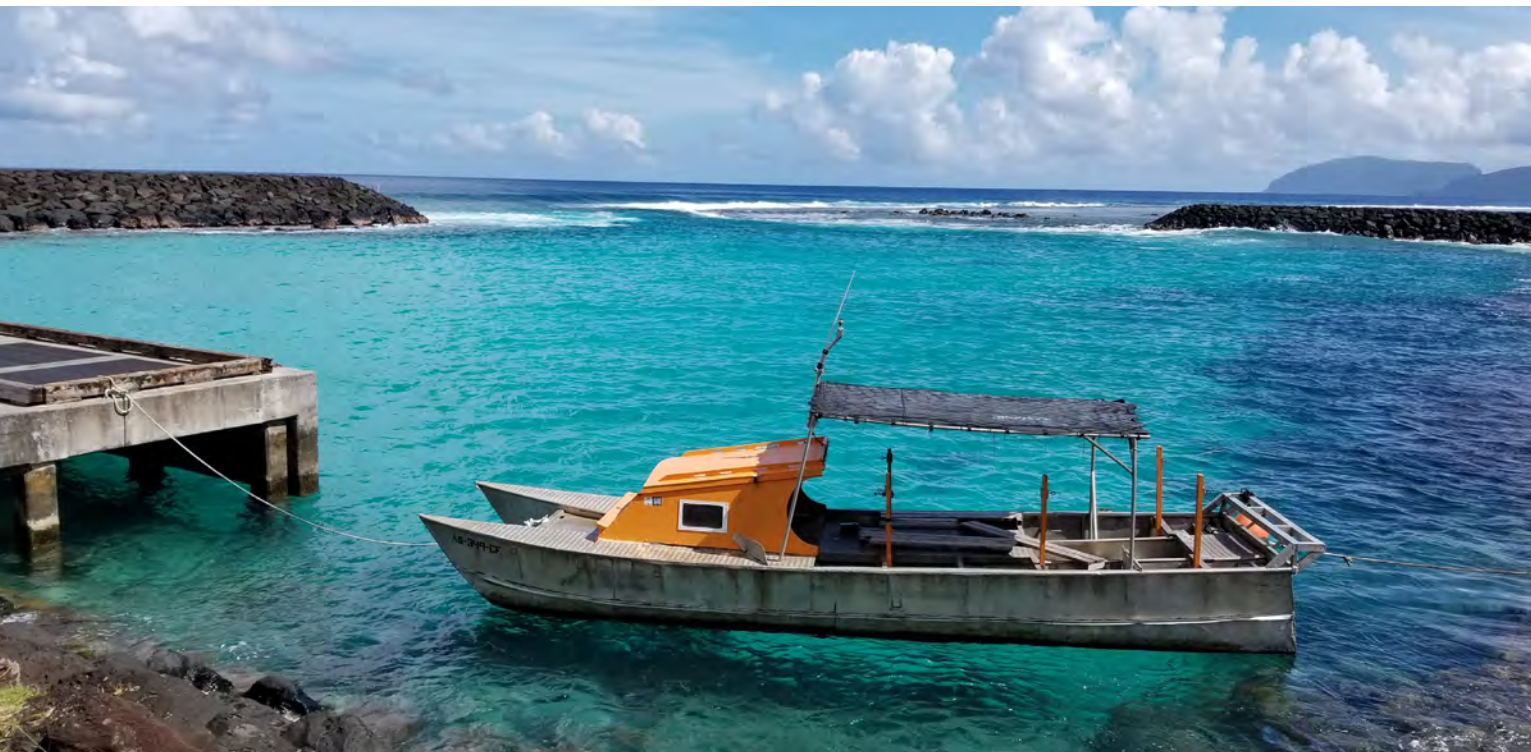
Alia are small, double-hulled catamaran multi-purpose boats. They are used for commercial and subsistence fishing (pelagic trolling and bottomfishing) or for transportation like the vessel seen in this photo taken at Ta'u Harbor, American Samoa. © Nate Ilaoa
