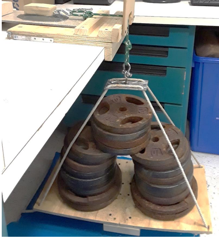
Figure 4.2. Side view of the force apparatus employed in full-scale testing with several 4.5 kg weights loaded onto bottom weight tray. Replicates were secured onto the force apparatus by a pivoting wooden block to a wooden surface with adjustable inclines. The weight tray was attached by rope and S-hook to eye-screws mounted in each experimental unit. Rope passed through a safety visor, which served to protect researchers during trials.
