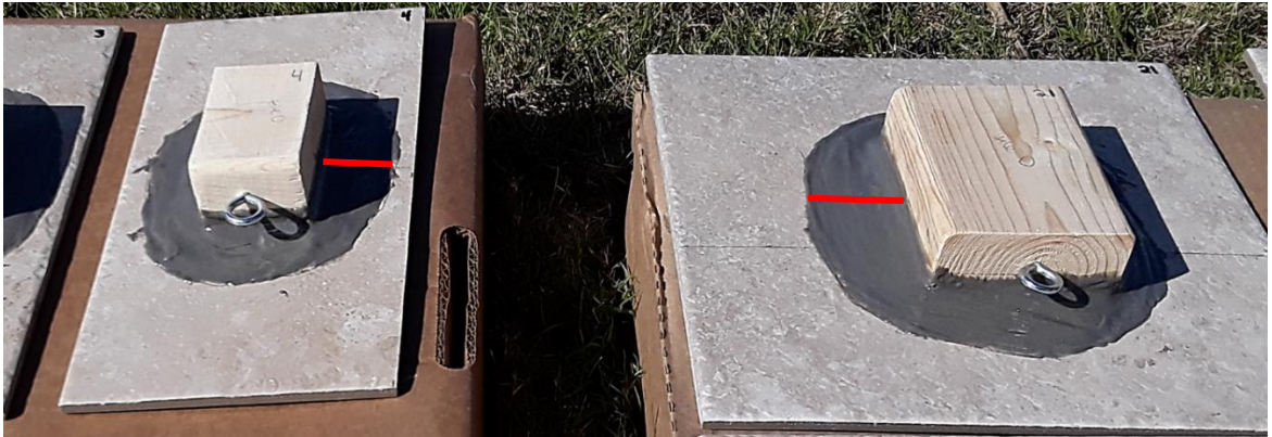
Figure 4.1. Experimental units with small (left) and large (right) surrogate transmitters affixed to tile 1. Small wooden blocks correspond to SPOT and TAM-4310 transmitters; large blocks correspond to ST-20 and TAM-4525 transmitters. Epoxy extends in four cm arc beyond edge of block, denoted by red lines.
