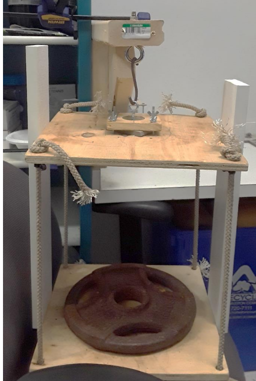
Figure AC.1. Front view of the force apparatus employed in small-scale testing with one 4.5 kg weight loaded onto bottom weight tray. Replicates were secured onto force apparatus by a wooden brace with a circular cut-out measuring 3.6 cm in diameter, and mounted by eye-screw.
