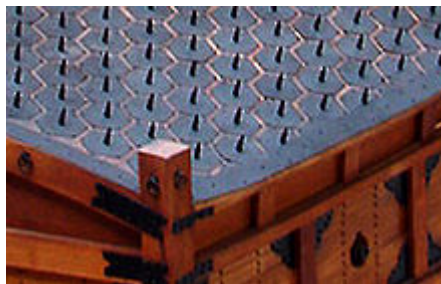
Deck Spikes on the Turtle Ship in the War Memorial of Korea museum
