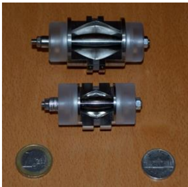
Figure 1.2. Two Orbitrap analyzers with both a 1-Euro coin and an American nickel as a reference for size [24]. The smaller device is the newer ultra-high resolution Orbitrap analyzer.
