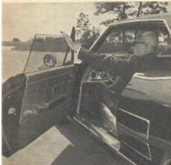
Windows without frames were made possible by redesigning the Buick's outer door panels.
