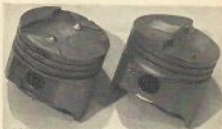
For better combustion, Continental swaps old piston (left) for half-wedge-top type.
