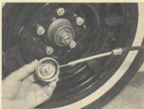
Shades of yesteryear! Photo shows spindle on lugs side of wheel, speedometer cable, and mounting. Installation is on inside of wheel.
