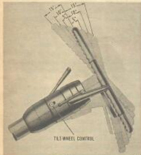
Tilting steering wheel lets you take your pick of seven positions for driving comfort.
