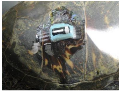
Figure 2. Attachment of Vemco V13-1L acoustic transmitter to the third lateral scute using a silicon elastomer base, fiberglass cloth and polyester resin. Note the one end of the tag was left uncovered so that sonic transmissions could occur.
