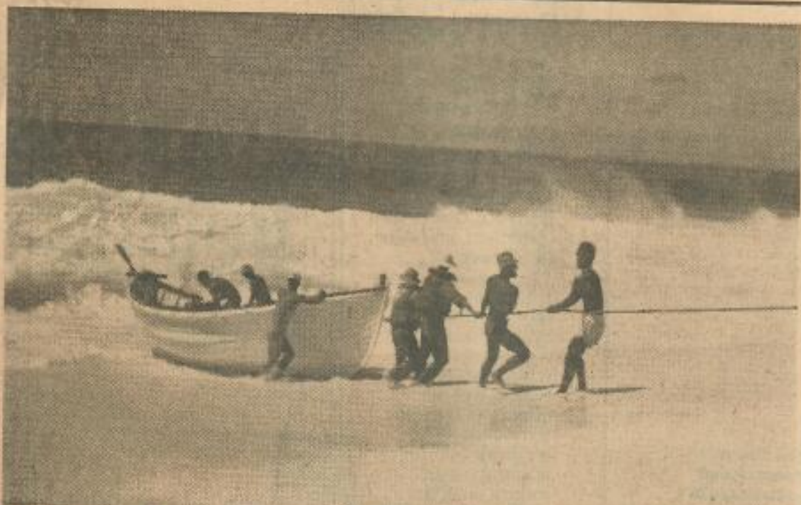
Landing men and supplies on Howland Island: In dangerous surf a towline was used to haul a longboat between the beach and waiting boats offshore.
