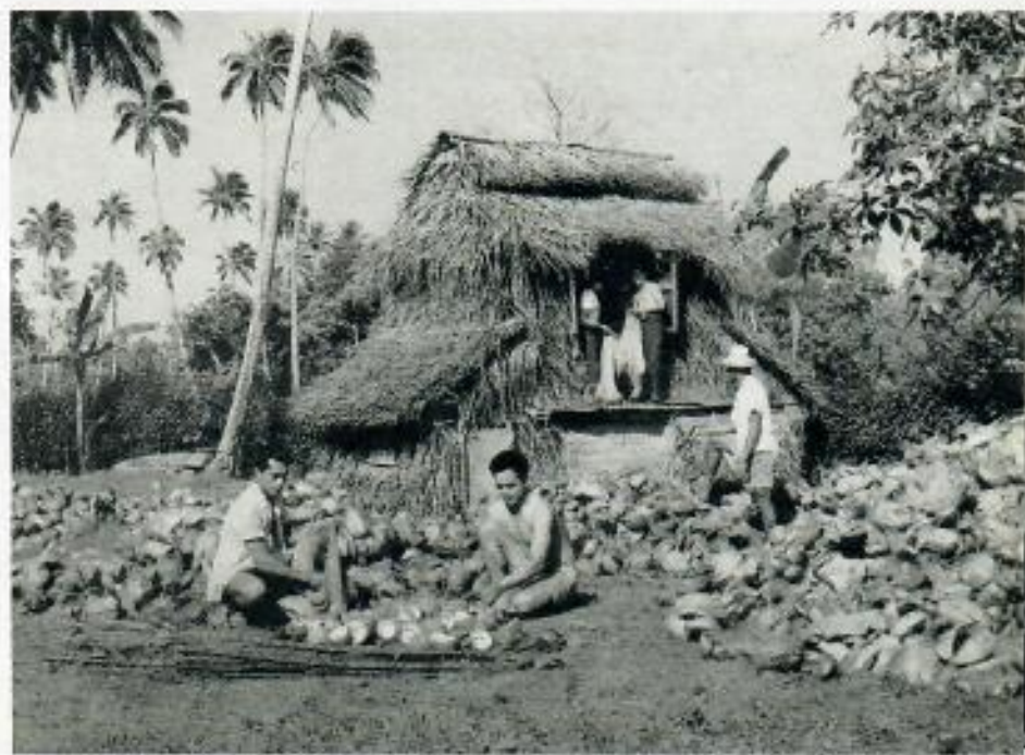
Cheaply-built copra driers, fueled mostly by waste husks, produce better quality and higher prices than sun-drying methods which are affected by rain.
