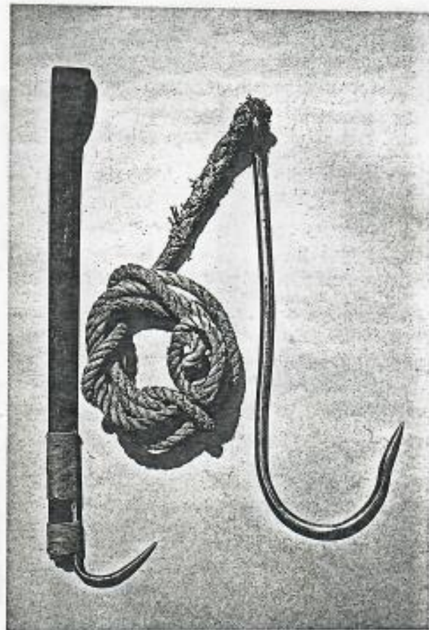
61. Gaffs for boating large fish. The lower one is a flying gaff used for boating marlin.
