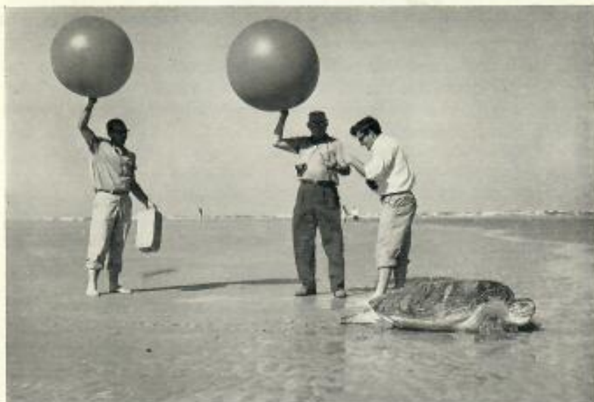
FIG. 1. The rig used in balloon tracking tests. The styrofoam float (held by man at left) was fastened to the hind edge of the shell with 30 ft of monofilament line. Two balloons rose on 10 and 15 ft lines. The tow-line swivel was attached to the shell with thin iron wire, designed to rust away within a short time and free the turtle of the rig. All turtles tested were marked with standard fin tags.
