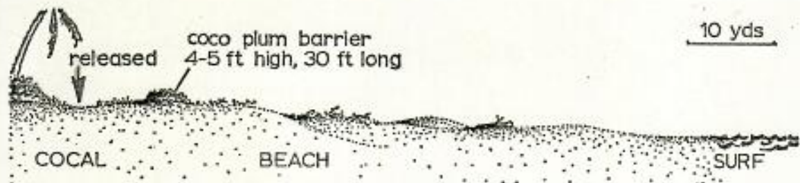
FIG. 15. Beach profile, showing conditions of test 13.
