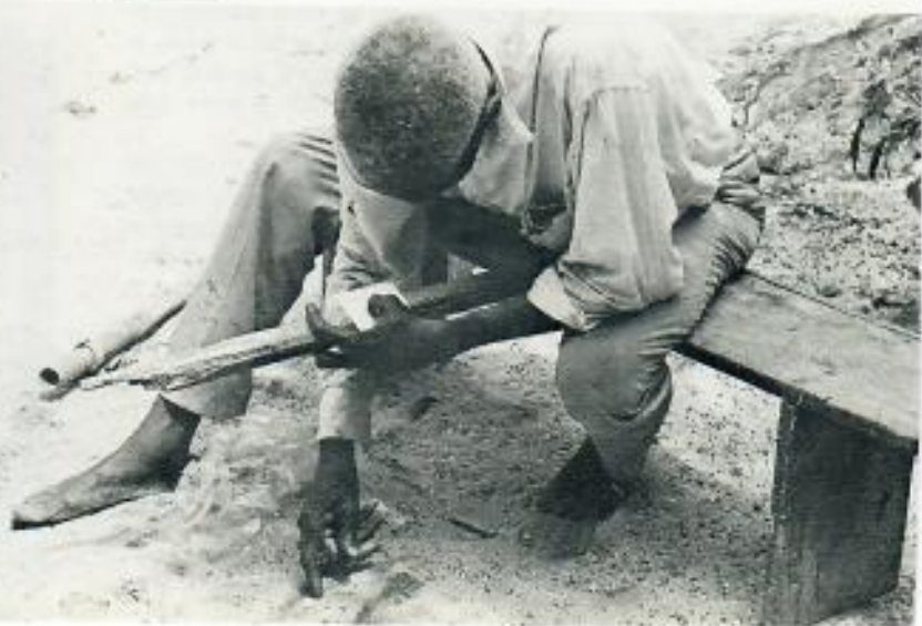
LEFT (TOP AND MIDDLE): Ellsworth Ebanks demonstrates the making of lead ball weights. A nail is pushed through the mould, then molten lead poured in, held for a few seconds then dropped into cold water to harden. This mould has been used by several generations of the Barnett family. TOP RIGHT: Bernel Dixon displays lead weights threaded on to a line. BOTTOM LEFT: Closeup of a cast net shows how the lead balls are placed at equal distances along the footrope. BELOW: Bernel demonstrates on the sand how to make a needle.
