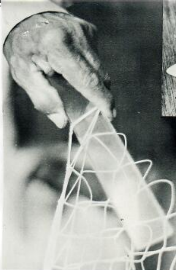
LEFT: Zacarias Christian uses a former, which he made out of plexiglass, to ensure that all meshes of a net are the same size. ABOVE: A "needle" loaded with the twine from which nets are made. This needle was made by Bernel Dixon.
