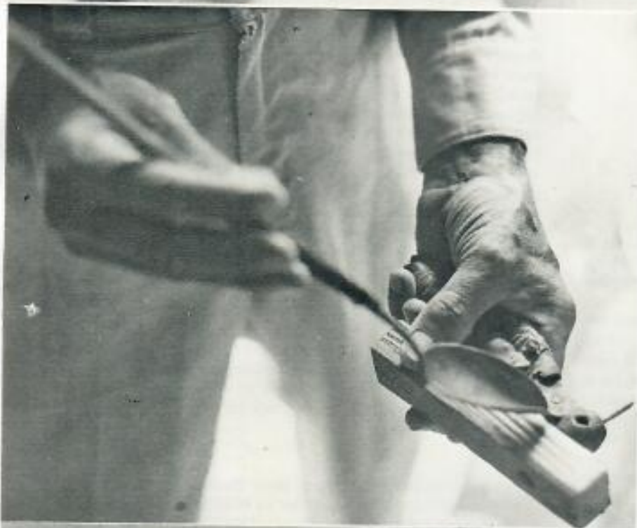
LEFT (TOP AND MIDDLE): Ellsworth Ebanks demonstrates the making of lead ball weights. A nail is pushed through the mould, then molten lead poured in, held for a few seconds then dropped into cold water to harden. This mould has been used by several generations of the Barnett family. TOP RIGHT: Bernel Dixon displays lead weights threaded on to a line. BOTTOM LEFT: Closeup of a cast net shows how the lead balls are placed at equal distances along the footrope. BELOW: Bernel demonstrates on the sand how to make a needle.
