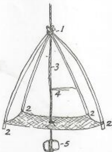
FIGURE 277.—Baited net ( ʻūpenya sumu ): four thin rods about as thick as a lead pencil and 21 inches long were tied together (1) with sennit. A piece of two-ply sennit cord was then threaded through the marginal meshes of a rectangular piece of net 17 inches long by 15.5 inches wide and tied with a clove hitch round the lower end of each rod (2). Another piece of cord (3) was tied to the top of the handle (1) and passed down through the middle of the net. A piece of thread was used to tie the cord to a net mesh where it passed through. Another thread (4) was tied to the cord above the net for tying on the bait of a piece of coconut meat or crab. A stone sinker (5) was tied to the cord below the net. From the upper end of the rods (1) to the net was about 16.5 inches while the bait thread was 5 inches above the net.
