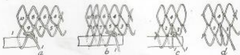
FIGURE 273.—Netting technique and additional meshes: a and b , increasing length; c and d , additional meshes. a , The net strip from the position in figure 272 d is now laid transversely with the cord on the left and the pull being changed the appearance is as shown. The gage is placed over the cord (1) and the first mesh made by engaging with the mesh (9). The first mesh formed has a free margin formed by the cord descending to the upper edge of the gage and passing behind it. b , When the first mesh of the new row is tied, it is not now necessary to remove the gage from it. The gage is simply pushed along under the next completed mesh above. From now on, it will be noted that the last knot tied is on the upper edge of the gage. The cord (1) is simply passed behind the gage brought up over the lower edge, the needle passed through the next mesh (3) and the usual knot made. Thus after the first marginal mesh of the new row, each mesh is formed by the sides of the meshes above while the cord simply adds the lower half of the mesh. The same number of meshes are made as in the row above. The netting is then twisted over to bring the cord back to the left and another row commenced. The successive rows are added until the length required is finished. See Plate XLV, A , 3. c , Instead of carrying the cord (1) from the last knot (2) to the next mesh loop (3), the needle is passed through the loop above (4). The cord is brought down to the mesh gage and tied to the ascending cord with the usual netting knot as shown. d , The needle is now passed through the next mesh (3) and the netting knot tied. Thus between the knots (2) and (3) there are two meshes instead of one.
