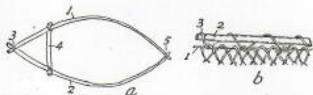
FIGURE 275.—Frame and net attachment of 'upenga sae'e : a, the frame is formed of 2 rods (1, 2) tied together at the thicker ends (3). A crossbar (4) about 12 inches long is lashed to the side rods about 8.5 inches from the lashing (3) to spread them. The rod ends are brought together about 28.5 inches from the crossbar and tied (5). The frame is 16.5 inches across at its widest part. b, A bag net with a line (1) threaded through the marginal meshes of its upper circumference is attached to the frame (2) by another cord (3) wound spirally around the frame and the circumferential line. The net is 32 inches deep and narrowed longitudinally at the bottom to 23 inches.
