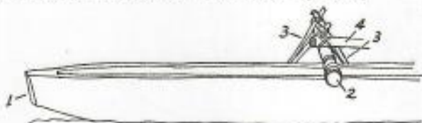
FIGURE 222.— Soatau dugout canoe, stern end: 1, square stern, no hauling knob; 2, aft boom; 3, two pairs connecting pegs, widely divergent lower ends, upper ends crossed over boom; 4, longitudinal pole lashed to booms to inner side of connecting peg lashings (after Kramer).
