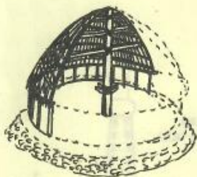
FALE UNDER CONSTRUCTION
