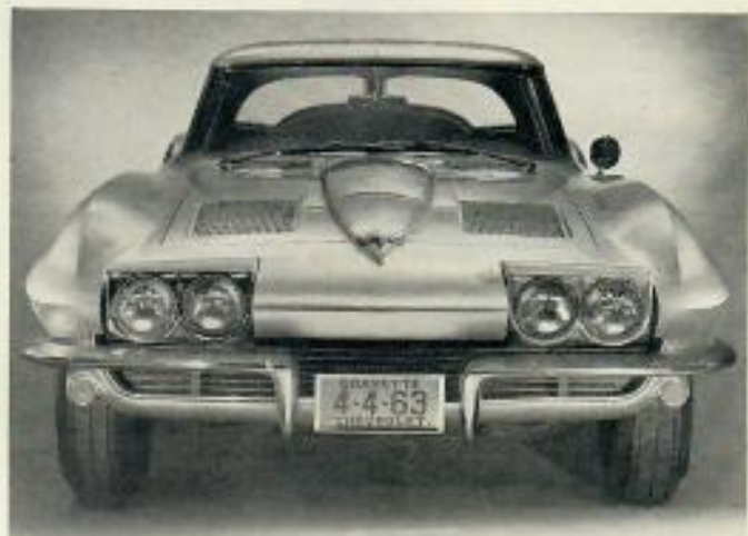
The headlight buckets are rotated into operating position by electric motors—with stops for correct height adjustment.
