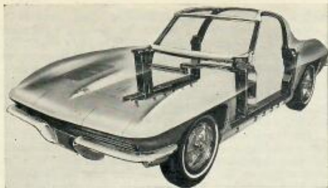
Steel reinforcing is built into the coupe body.
