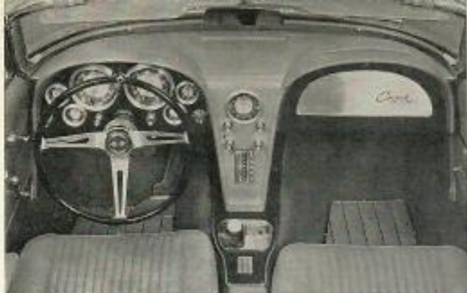
Cockpit changes, above, are many. Note the carpet inlays and "grab-bar" incorporated in the right dash nacelle trim.
