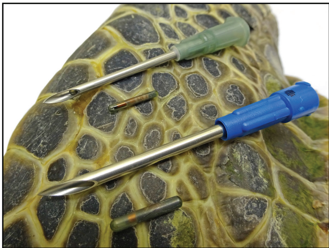
Figure 1. Relative size of PIT tags and associated implantation needles and the proximal front flipper of a juvenile green turtle ( Chelonia mydas ). Shown are a 16-gauge needle and a 10.3 mm PIT tag (MiniHPT10, top) and a 12-gauge needle and a 12.5 mm PIT tag (ATP12 PL, bottom)
