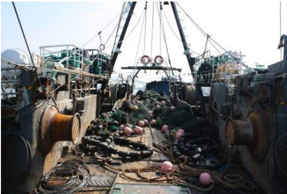
12. A vessel of Nisou-biki which is a kind of trawls operated by 2 vessels in Sakaiminato, Tottori.
