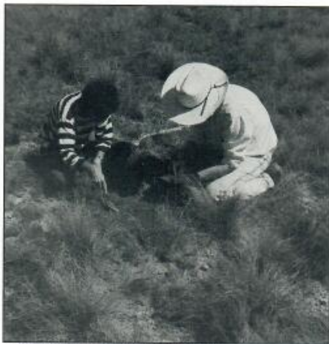
Photo 3. Conducting trowel test of soil
