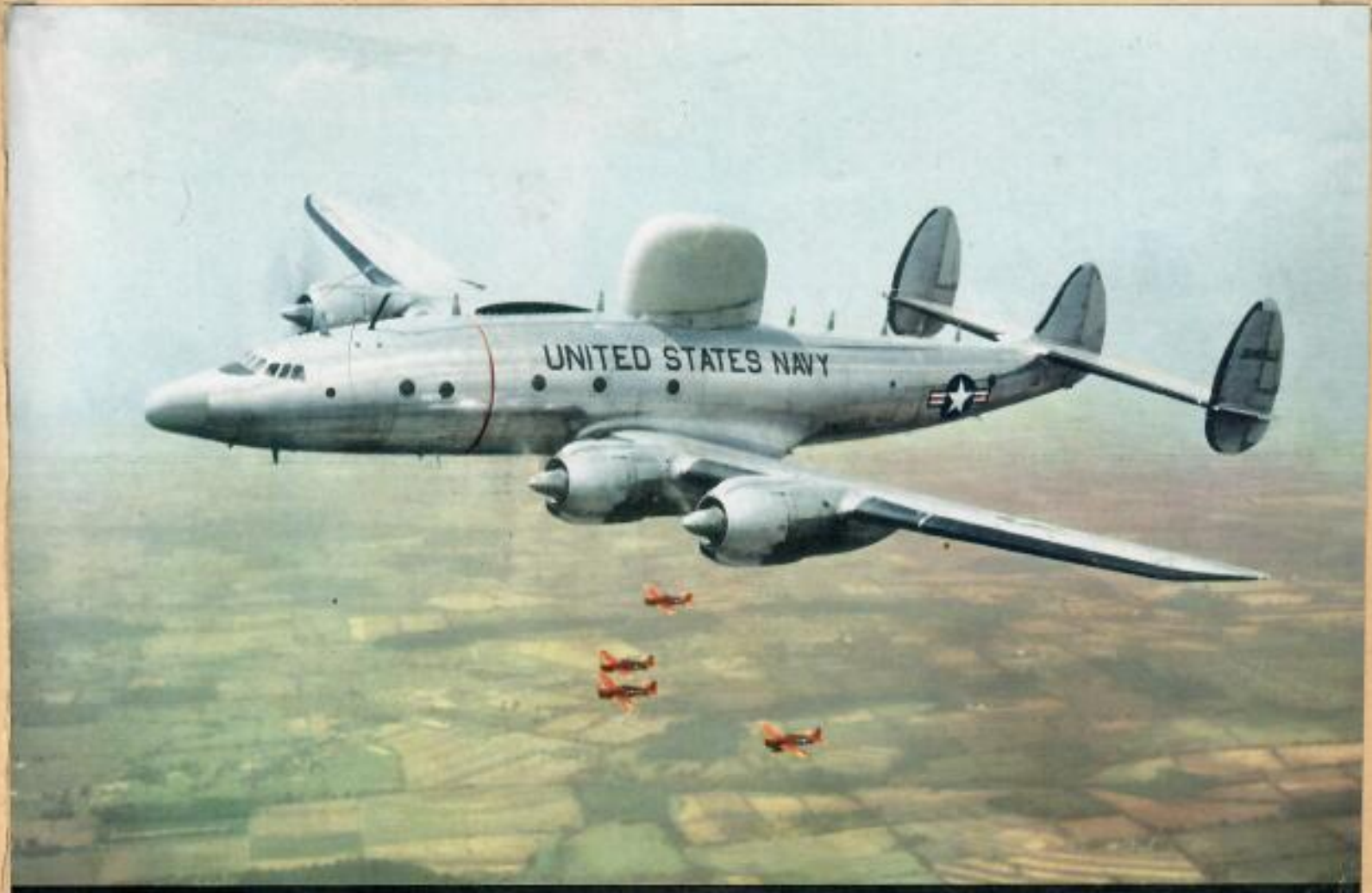
PO-1W Constellation tests electronic systems for Naval planes. Note plane's radome and drones below.
