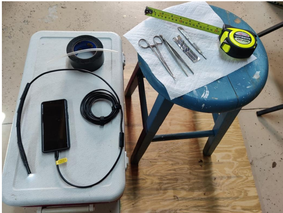
Figure 1. AnyKit Endoscope (borescope) system. From left, modified scope attached to phone. Our scope has been modified with a section of tigon tubing then covered with waterproof tape. Above is a separate section of tigon tube and the type of tape used to cover the cable to make it stiffer. Also shown are the instruments (hemostat, forceps, rounded blade #10 and scalpel #3) and lab stool for holding turtle in an inverted position.
