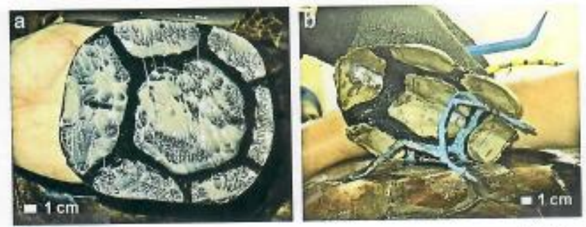
Fig. 3. Epoxy pattern on neoprene removed (a) immediately after attachment and (b) at the end of Trial 2.
